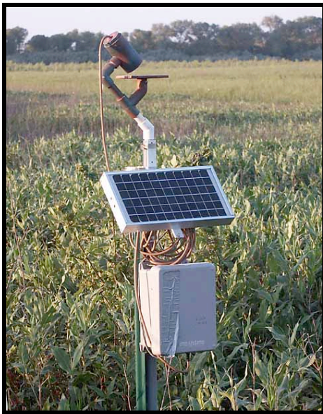
Figure 5. Solar powered bat ultrasound monitor on the Lower Floodplain.
